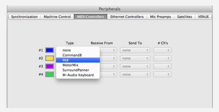
3. Set the Receive From and Send To options to "Faderport". # Ch's should be set to 8. Click Ok.
