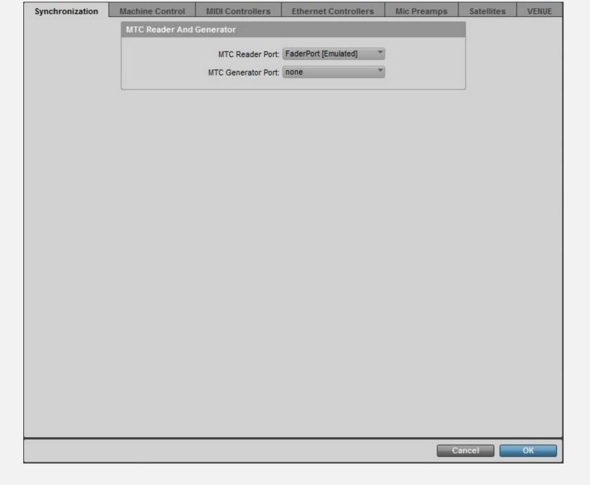
MIDI Machine Control should be enabled to read "Faderport [Emulated]" with default values selected.
